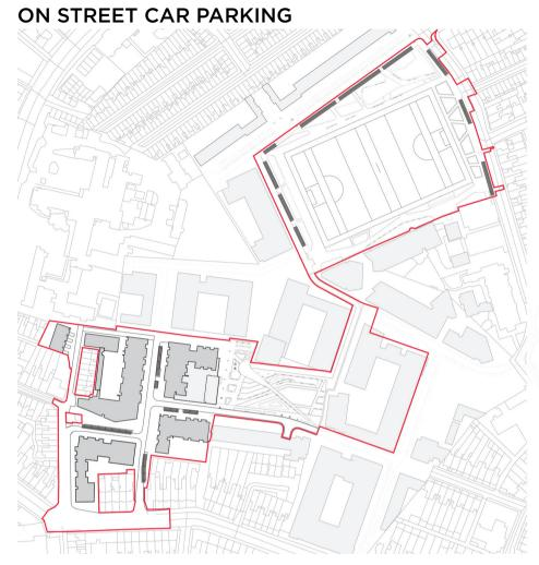
Materials for street car parking will be delineated in a contrasting concrete or natural stone paving unit 100mm x 100mm or 100mm x 200mm. Finishes will be bush hammered with slip resistance to meet local standards and compressive strength to handle service vehicle run over. Tones will vary with surrounding materials.
