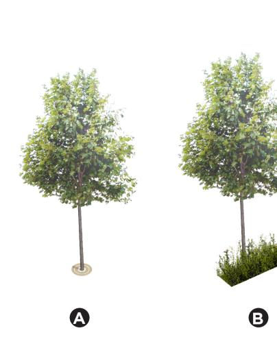
Type A: Covered tree pit with connecting trench. – Typical Soil Volume = 6m3 excluding trench and 8.5m3 including trench – Drained Area typically 30-50m2 per individual tree pit Type B: Open tree pit with connecting trench. – Typical Soil Volume = 5.7m3 excluding trench and 7.5m3 including trench – Drained Area typically 30-50m2 per individual tree pit
