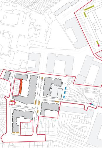
A variety of edge and boundary treatments have been proposed (reference L1-104 Boundary Conditions Plan) .The existing boundary walls maintain their character where possible while the new boundary features replicate the traditional pattern of the immediate locality with respect to scale and material.
